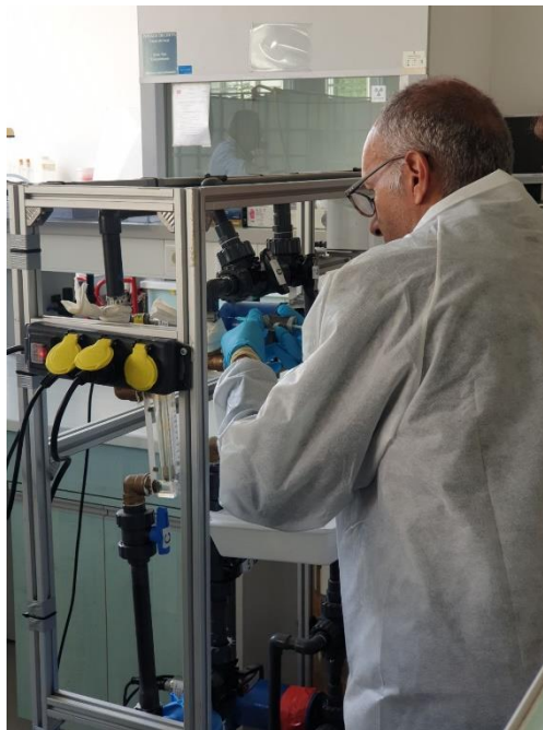
Figure 2. Injection of Radiotracer for Flow Rate Measurement Experiment
