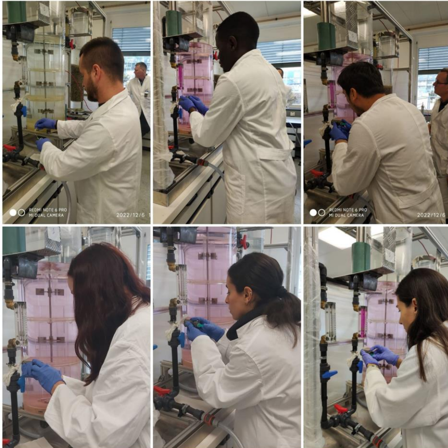
Figure 4. Injection of radiotracer by participants
