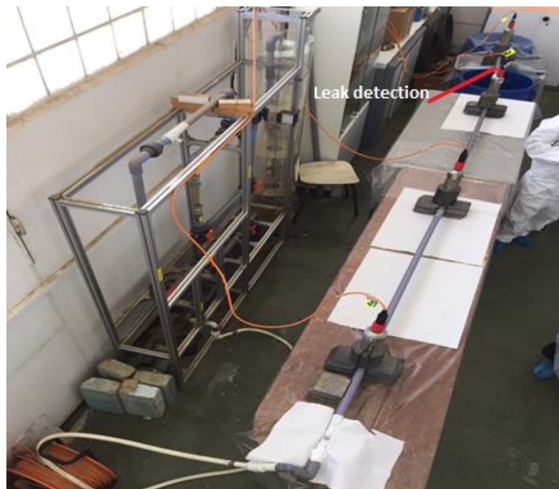
Fig. 1 Experimental setup for radiotracer measurements in pipes
