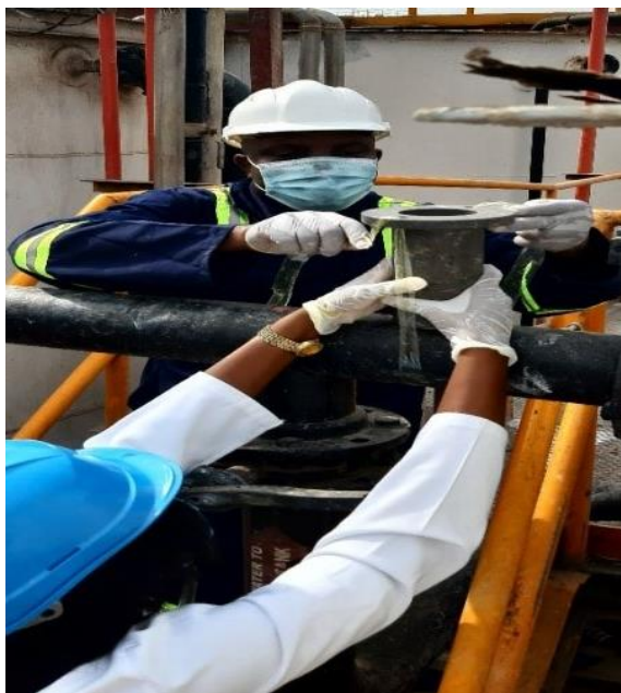
Fig. 1. Mounting of detector collimators (left) and background radiation counting initiation (right)
